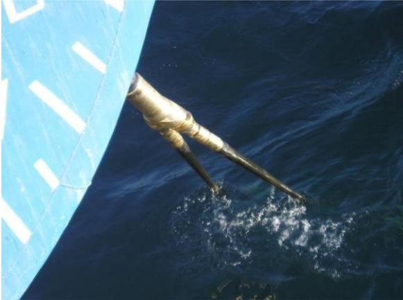
**Figure 4** Branching Unit for MINISUB™ repeaterless submarine cable being deployed in the North Sea
