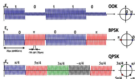
**Figure 1: OOK, BPSK and QPSK modulation**
