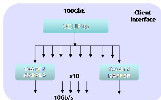
Figure 5: 100GbE client interface architecture
