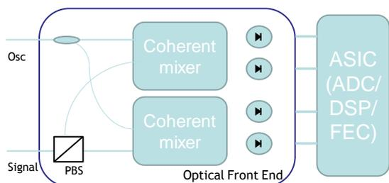
**Figure 2: Coherent receiver**
