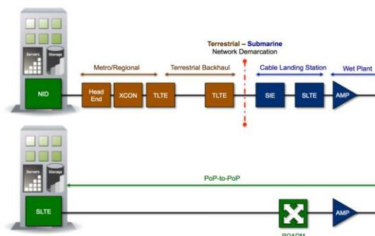
Figure 3: Cable Landing Station simplification leveraging *Optical Bypass* architectures
