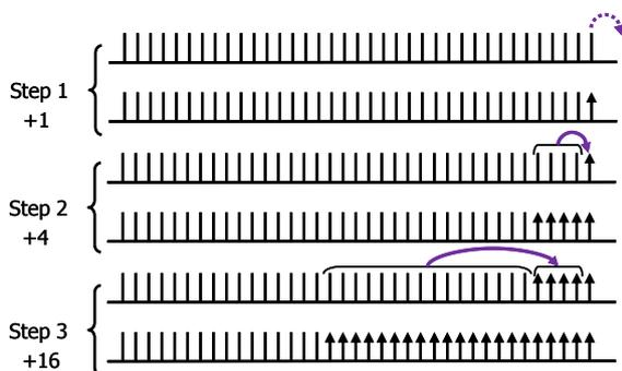
Figure 2: Spectral representation of the step by step capacity increase with traffic migrations. New waves are represented by an arrow.
