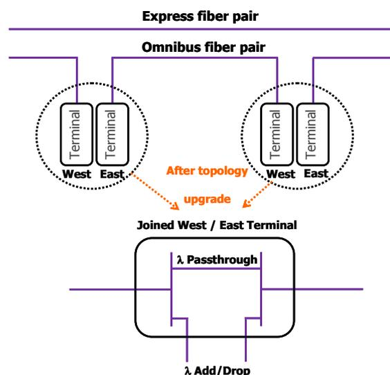
Figure 3: Moving to a wavelength passthrough in intermediate stations
