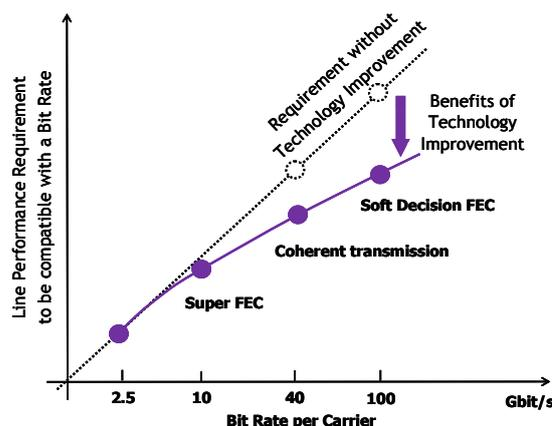
Figure 1: Upgradability of installed systems thanks to technology improvement
