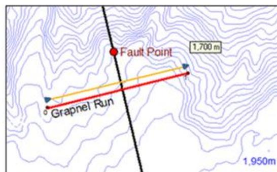
**Figure 4: CRM plan view display showing a grapnel run route.**
