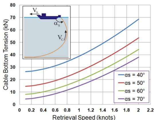
**Figure 2: Steady-State cable bottom tension vs. retrieval speed for light weight protected cable (4 N/m, 43 Knot-deg) being recovered from a depth of 2000 m.**
