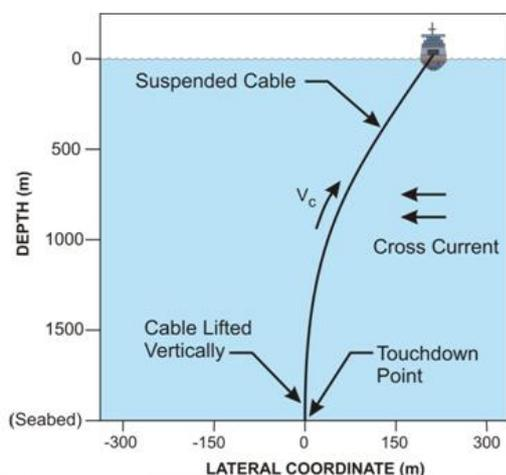
**Figure 3: Ideal configuration for cable recovery in the presence of cross currents.**
