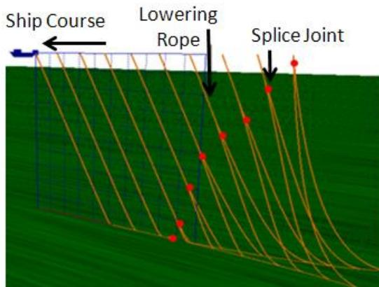
Figure 5: CRM display showing a splice joint being lowered.
