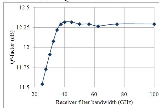
Figure 2: Impact of receiver filter bandwidth on one 40 Gb/s channel
