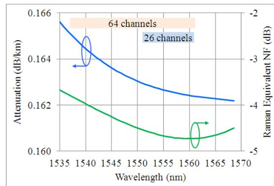
Figure 1: Evolution of fiber attenuation and Raman NF versus wavelength.
