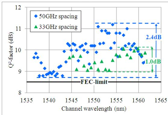
Figure 5:  $Q^2$ -factor for 64 x 40 Gb/s transmission with 50 GHz and 33 GHz channel spacing
