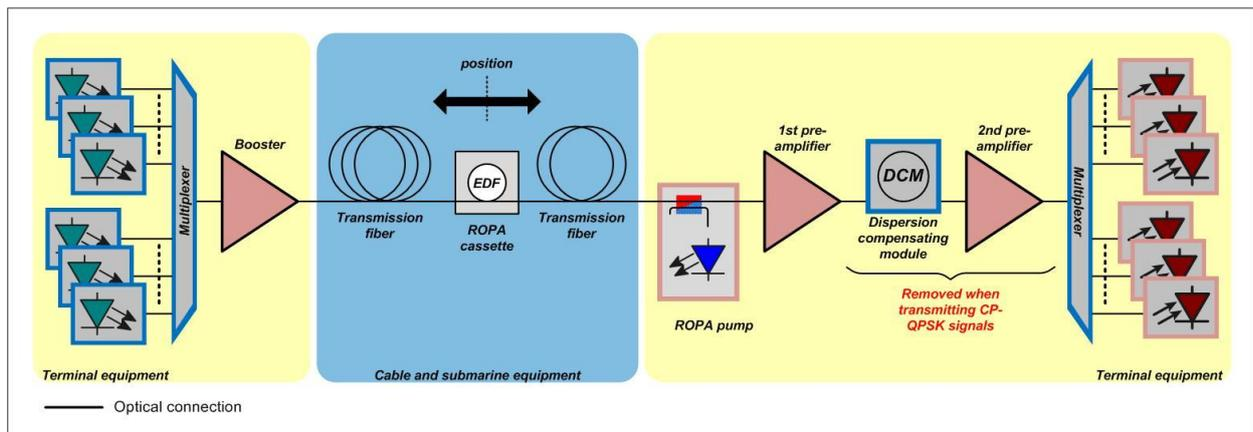
**Figure 1: Setup of the investigated long single span system for submarine applications**
