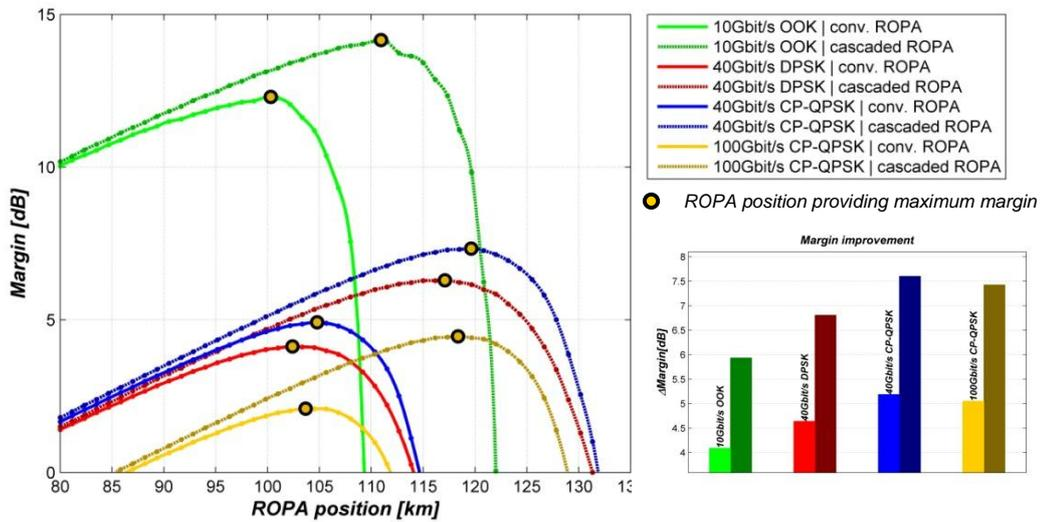
**Figure 2:** *Left side:* OSNR margin versus ROPA position for different modulation schemes and ROPA types for a WDM system with 20 channels. *Right side:* OSNR improvement for conventional ROPA (left bar) and cascaded ROPA (right bar) for different modulation schemes.
