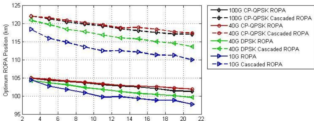
**Figure 3:** Optimum ROPA position as a function of number of channels for different modulation schemes and ROPA types
