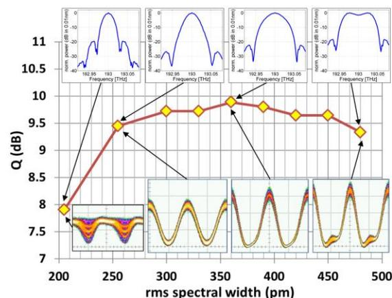
Figure 2: Q factor as a function of the spectral rms width of the DP-QPSK signal. Insets show pulse shapes and spectra before optical filtering.
