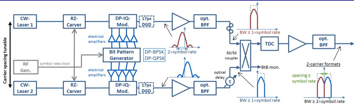
**Figure 1: Schematic of the test channel transmitter. (CW: continuous wave, RZ: return to zero, BPF: band pass filter, TDC: tunable dispersion compensator)**
