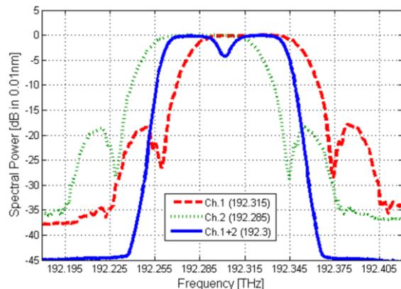
**Figure 4: Resulting spectra of the dual-carrier signals at the transmitter: Red and green spectra show the individual subcarriers after pulse shaping and blue spectrum is the filtered dual-carrier channel at the transmitter output.**
