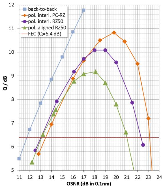
**Figure 3: Q-factor as a function of the received OSNR for different configurations on link #1.**
