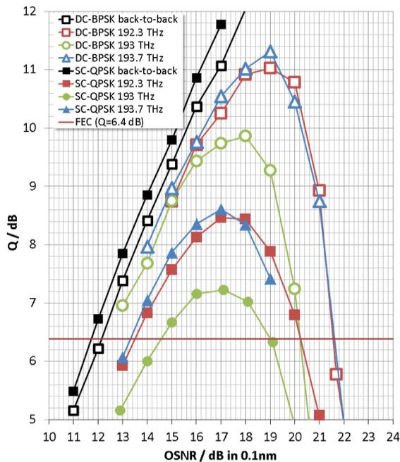
**Figure 5: Q-factor as a function of the received OSNR for link #2. Open symbols represent the dual-carrier configurations with separate detection of both subcarriers.**
