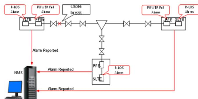
Figure 2 Fault diagnosis and locating on alarms
