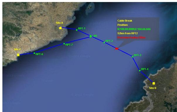
Figure 6 Demonstration of a cable break fault report
