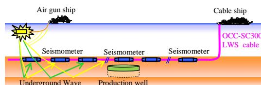
Figure 1: Configuration of the DSS
