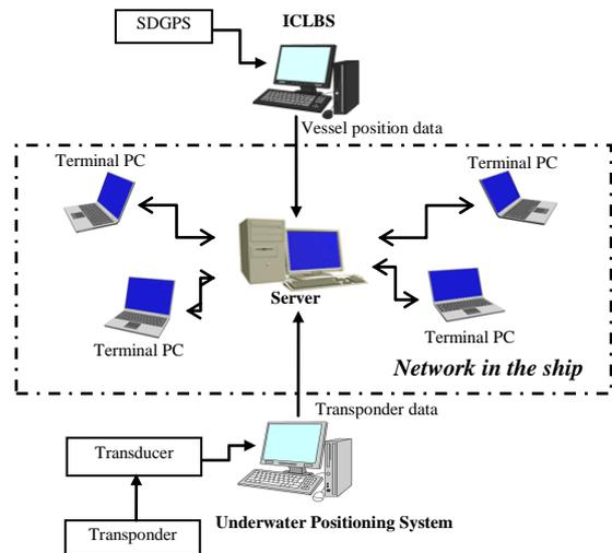
Figure 6: Configuration of real-time 3-D plotting system
