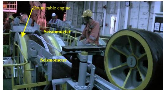
Photo 1: The seismometer on the drum cable engine
