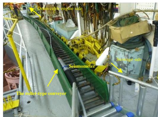
Photo 3: The seismometer on the conveyer
