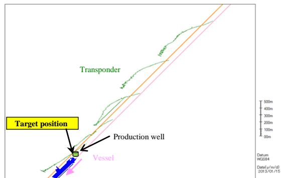
Figure 7: Track of the transponders during the deployment
