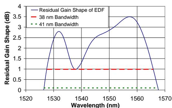
**Figure 3: EDF Gain shape to be corrected by the gain flattening filter (GFF), for 38nm (dashed line) and 41nm (dotted line).**
