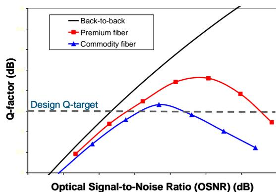
**Figure 1: Designs of a transpacific link with premium and commodity +D fiber.**
