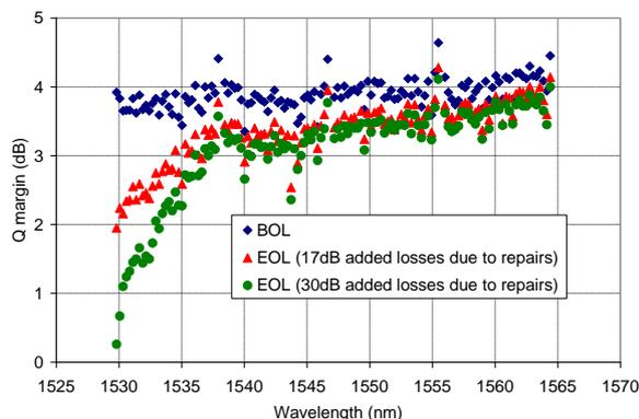
**Figure 2: Performance degradation as a function of added path loss.**
