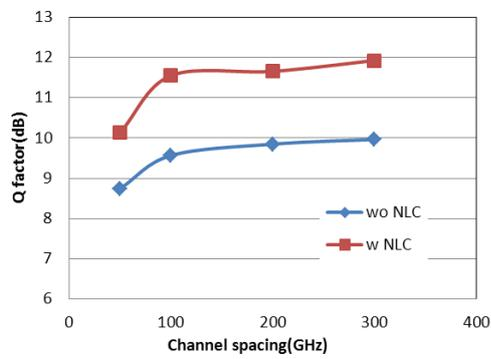
Figure 4.1 channel spacing dependence between 100G DP-QPSK and 10G OOK signal
