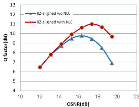
Figure 3.2 OSNR dependence of Q value after NZ-DSF 4000km-transmission (1559.794nm).
