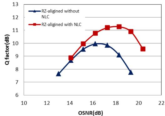
Figure 3.7 OSNR dependence of Q value after DMF 6,000km-transmission (1550.114nm).
