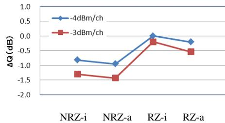
Figure 3.3 Q factor without NLC ( $\Delta Q$  is normalized at Q factor of RZ-i without NLC at -4 dBm/ch )
