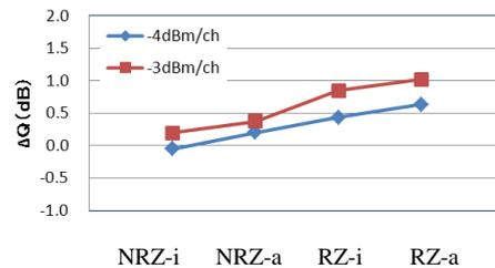
Figure 3.4 Q factor with NLC ( $\Delta Q$  is normalized at Q factor of RZ-i without NLC at -4 dBm/ch )
