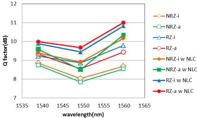
Figure 3.5 channel dependence of Q value
