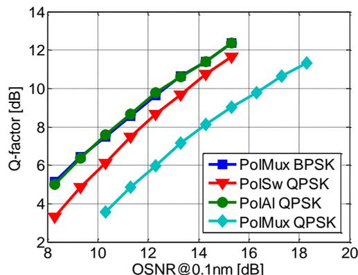
Figure 4 : Measured back-to-back Q-factor of different signals versus OSNR at 0.1 nm.
