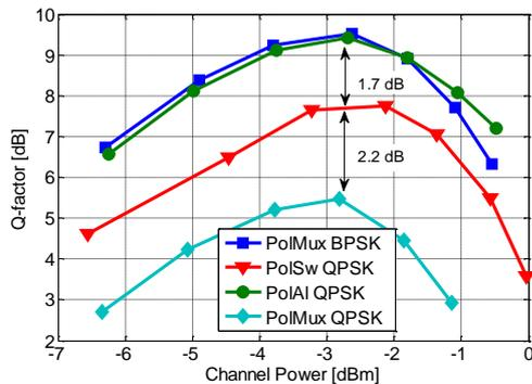
**Figure 5: The measured Q-factor as a function of channel power at 12 loops.**
