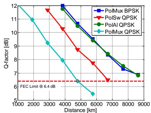
**Figure 6: Q-factor versus transmission distance at channel power of  $\sim -2.8\text{ dBm}$ .**
