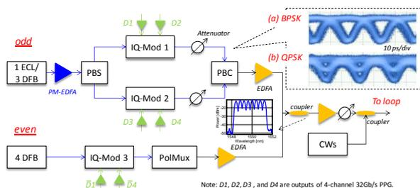
Figure 2 : Experimental setup for evaluating the flexible bit-rate transmitter.
