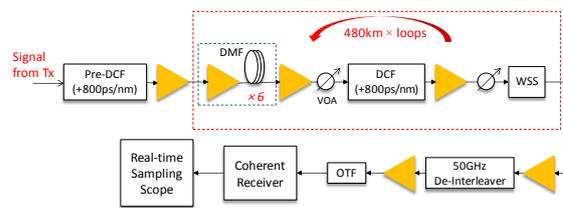
Figure 3 : Transmission link and receiver setup. OTF: optical tunable filter; VOA: variable optical attenuator.
