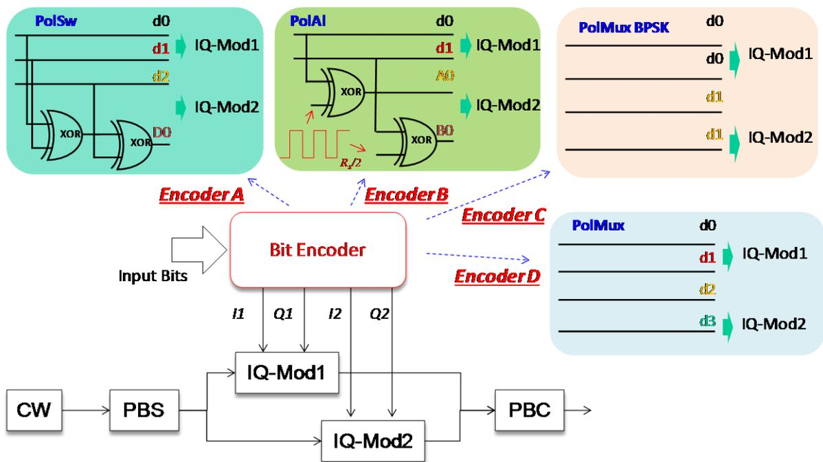
Figure 1 : The architecture of the proposed flexible transponder with four bit encoding modes for generating different polarization multiplexed signals.
