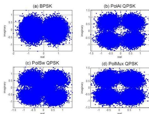
**Figure 6: The recovered constellation of (a) PolMux BPSK after 16 loops; (b) PolAl QPSK after 16 loops; (c) PolSw QPSK after 12 loops; and (d) PolMux QPSK after 8 loops.**
