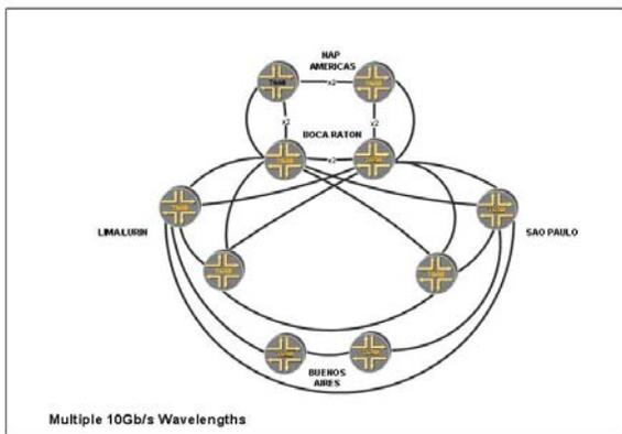
FIGURE 3 IP NETWORK OVER WDM LAYER
