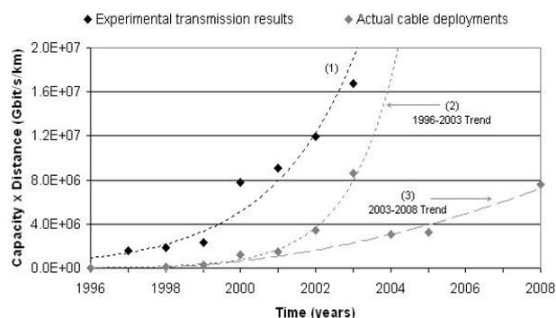
Figure 1 Laboratory results vs. designed capacity for actual cables (limited to C-band EDFA transmissions)
