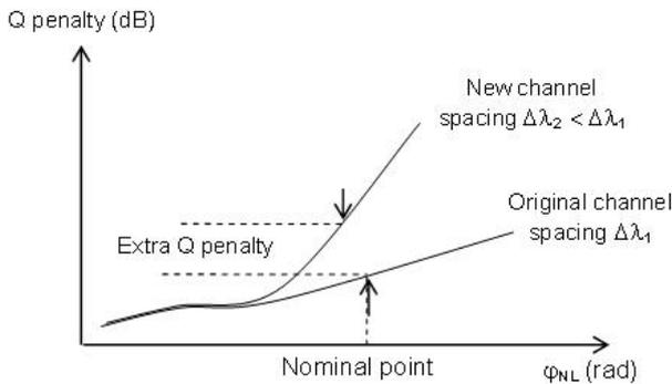
Figure 4 Q penalty as a function of the nonlinear phase noise and the channel spacing
