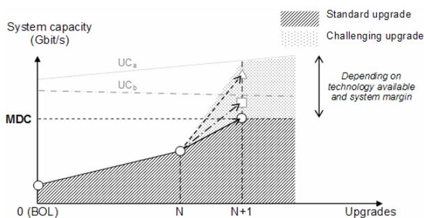
Figure 2 Upgrade and capacity definitions.  $UC_a$  (resp.  $UC_b$ ) is UC when replacing (resp. keeping) the existing equipment.
