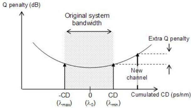
Figure 3 Q penalty as a function of accumulated CD for 10 Gbit/s OOK system
