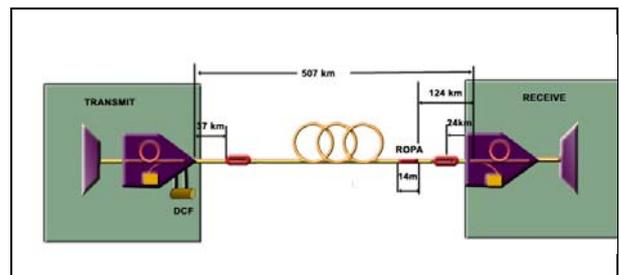
Figure 1: 507 Km Unrepeatered Set-Up
