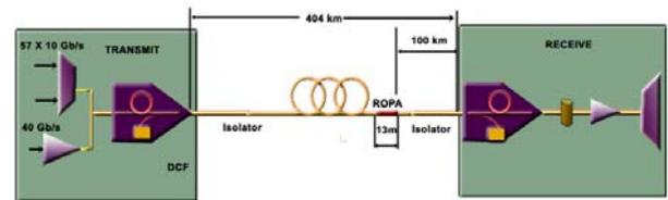
Figure 4: High-Capacity Unrepeatered demonstration set-up
