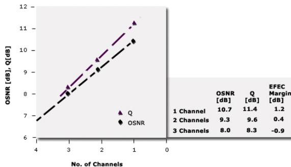
Figure 3: Q, OSNR vs No of Channels
