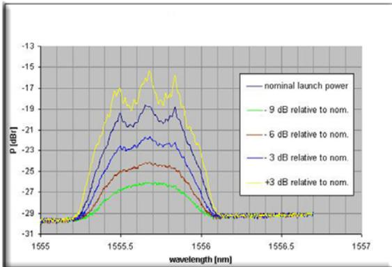
Figure 5: Non-Linear Distortion vs. Launch Power
