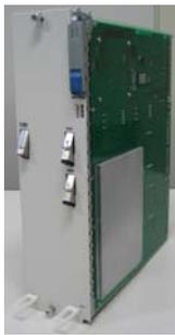
Fig. 9. Front View of 43Gb/s Transponder
