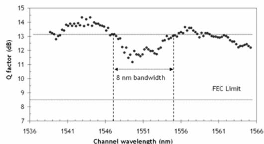
Fig. 4: Q factor measurements of 100 x 10 Gbps RZ-DPSK transmission with + 16 dBm EDFA output power
