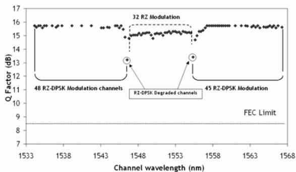
Fig.5 48 + 45 x 10 Gbps RZ-DPSK channels + 32 x 10 Gbps RZ-OOK channels, Q factor measurements - 4300 km NZDSF.
