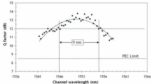
Fig. 3: Q factor measurements of 42 x 10 Gbps RZ-OOK transmission with + 12 dBm EDFA output power.
