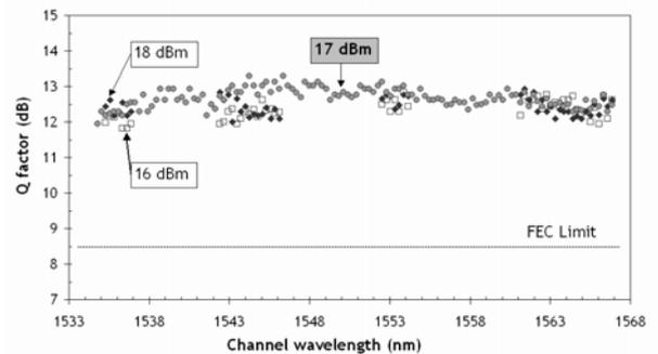
Fig. 1: Q factor measurements of 121 x 10 Gbps RZ-OOK transmission with +16 dBm, +17 dBm and +18 dBm EDFA output power.
