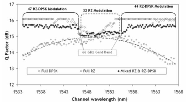
Fig.6 47 + 44 x 10 Gbps RZ-DPSK channels + 32 x 10 Gbps RZ-OOK channels, Q factor - 4300 km NZDSF.
