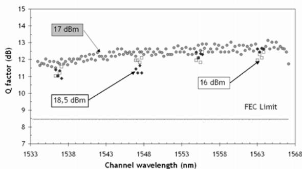
Fig. 2: Q factor of 125 x 10 Gbps RZ-DPSK transmission with + 16 dBm, + 17 dBm and + 18 dBm EDFA output power.
