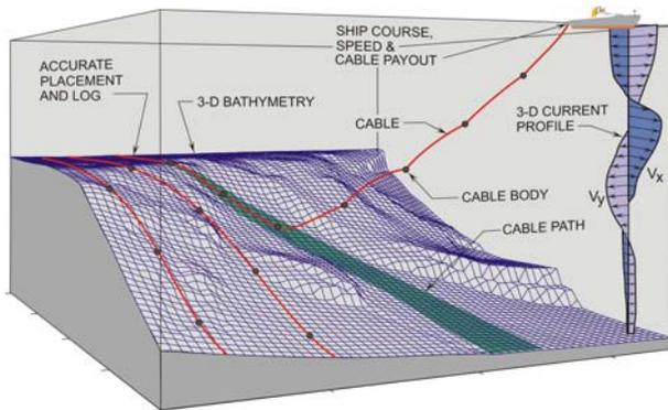
Figure 6. Factors affecting the 3D dynamic shape and touchdown conditions of a real submarine cable lay.
