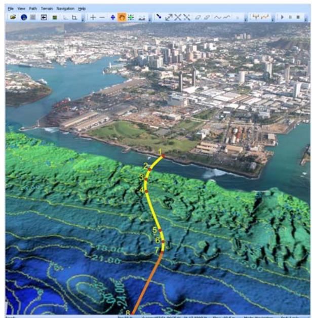
Figure 5. Visualizing and editing a cable route in a 3D, geo-referenced system.
