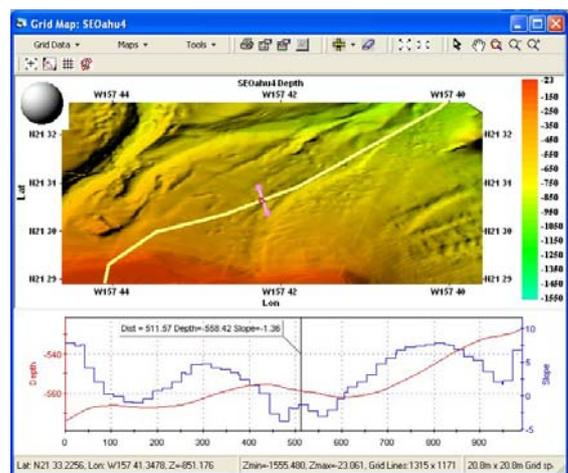
Figure 3. User can interactively create and modify the routes and reference lines, and depth profiles and slope graphs are automatically generated.
