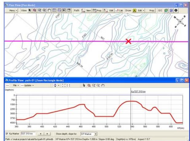
Figure 1. Cable route planners can now link plan and profile views to efficiently manage the cable route design process. Routes are edited using click and drag techniques and precise RPL and cable assembly lists and diagrams are created automatically.
