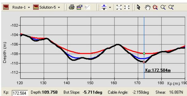
Figure 4. Example of cable suspension analysis for different tensions. This example shows the results of laying a cable over a section of the route (black line) using two different tensions. The final cable shapes are shown in red (for zero tension lay) and blue (for a higher tension lay).
