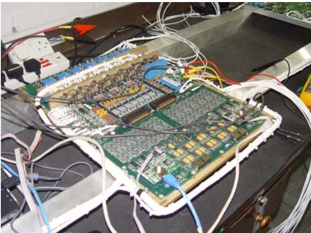
Fig 4: Elements of the LVPS being tested
