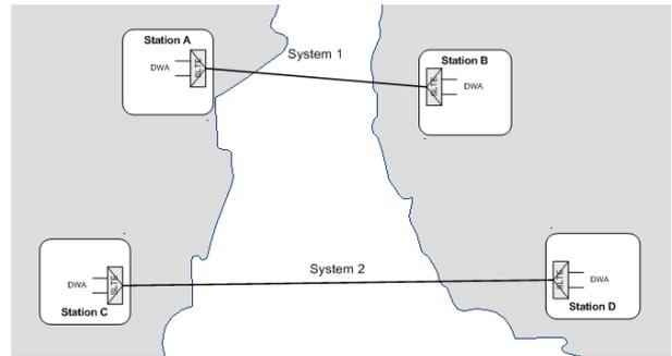
Figure 2: Direct Wavelength Access
