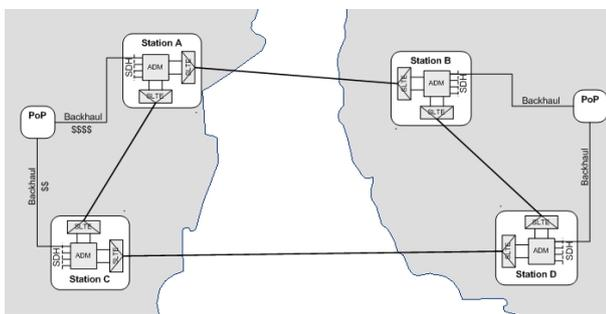
Figure 1: SDH-Based Ring System
