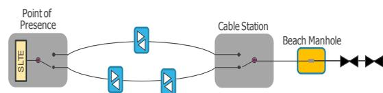
Figure 3 : Y Node protection scheme
