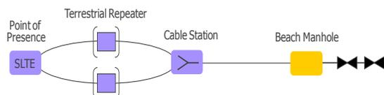
Figure 2 : Y Node Configuration
