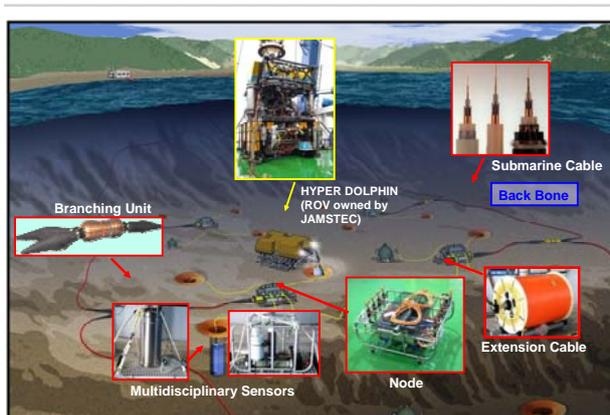
**Figure 3 Sample Node System Configuration (Courtesy of JAMSTEC)**
