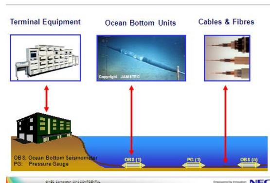
**Figure 2 In-Line System (typical configuration)**
