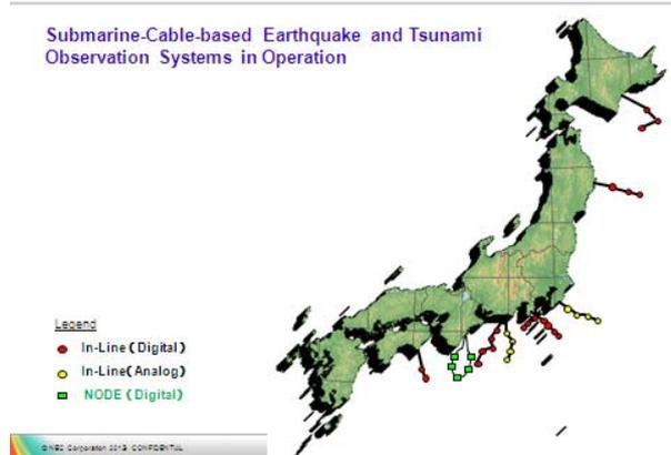
**Figure 1 Major Submarine Cable-based Observation Networks around Japan (NEC estimate)**
