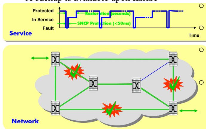
Figure 2: Protection and Restoration Combined (PRC)
