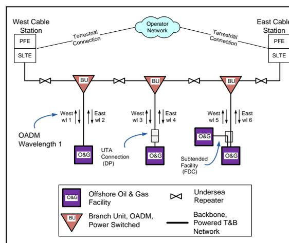
Figure 2: Powered Trunk and Branch OADM Offshore Network
