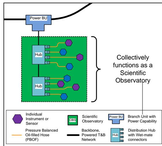
Figure 4: Hubs forming Observatory
