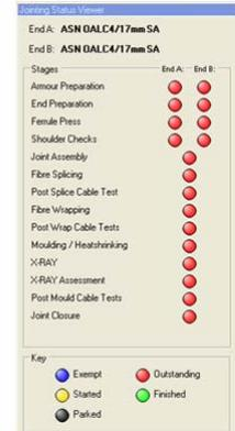
The Jointing Status Viewer has two functions. Not only does it indicate the status of the joint on the computer in the jointing area and also on separate computer screens elsewhere in the vessel, but it is also the Control Screen for JADE. By clicking on the appropriate buttons, sub-menus are displayed for starting, completing and parking the particular section. When the section is complete, the button changes colour to green.
