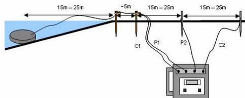
Continue to measure the resistance to Earth of the combined system of Copper Earth Spikes, Sea Earth Plate and Earth Leads
