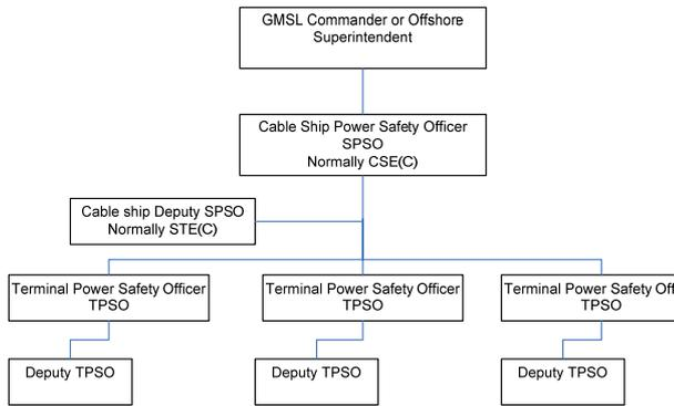
Figure 2 Power Safety Organisation for a cable ship. The CSE(C) and STE are Global Marine's in-house titles for the industry's equivalent of Chief Cable Engineer (CCE) and 2<sup>nd</sup> Cable Engineer
