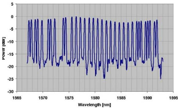
Figure 7: Egress amplifier normalized signal spectrum
