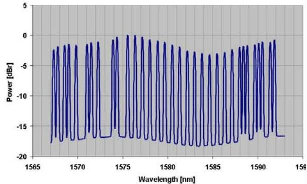
Figure 8: Pre-amplifier normalized signal spectrum
