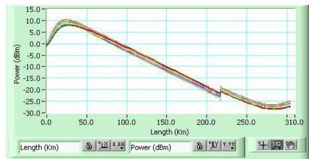
Figure 5: Simulated signal power profile along the link
