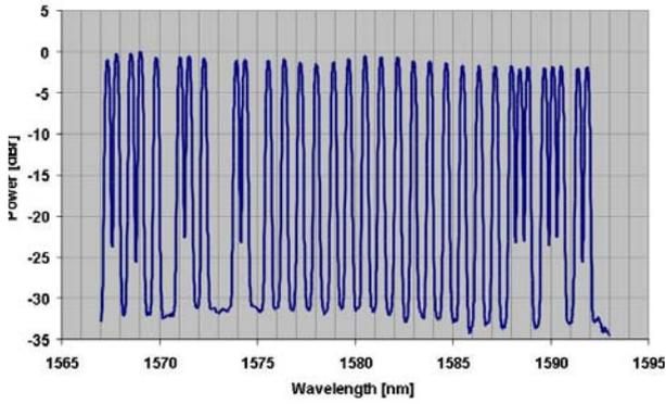
Figure 6: Ingress amplifier normalized signal spectrum
