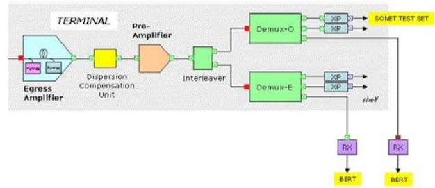
Figure 4: Raman receive terminal arrangement
