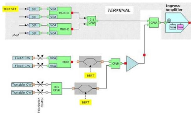
Figure 3: Raman transmit terminal arrangement
