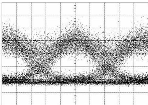
Figure 9: Received eye pattern @ 1592.10nm
