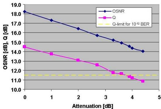
Figure 12: 1588.73 Performance as a function of attenuation
