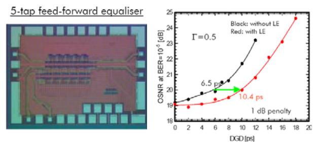
Fig 6: picture of EDE chip and experimental assessment of EDE efficiency to enhance PMD tolerance of modulation formats at 40Gb/s
