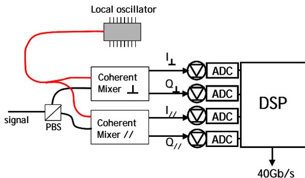
Fig 7 : scheme of coherent detection (can be applied to polarization multiplexed format).
