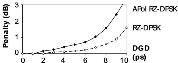
Fig 3 : tolerance to DGD of RZ-DPSK and APol RZ-DPSK
