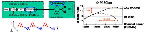
Fig 2 : left : evolution of transponder to evolve from RZ-DPSK to APol RZ-DPSK and impact on waveform. Right : Performance improvement brought by APol RZ-DPSK in a transpacific configuration
