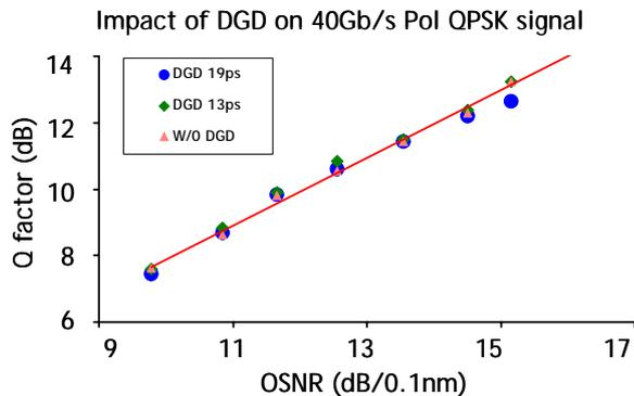
Fig 8 : Impact of DGD on OSNR sensitivity measurement of 40Gb/s Pol Mux QPSK signal
