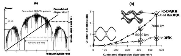
Fig 4 : left : Cumulated dispersion variation inside the RZ-DPSK spectrum. right : Q factor penalties consecutive to the impact of the cumulated dispersion slope inside a channel for both DPSK and RZ-DPSK formats. Insets : RZ-DPSK eye diagrams in back-to-back and after a dispersion slope degradation over 7000 km
