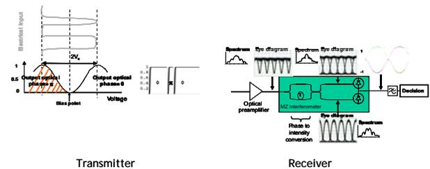
Fig 1 : DPSK transmitter (left) and receiver (right)
