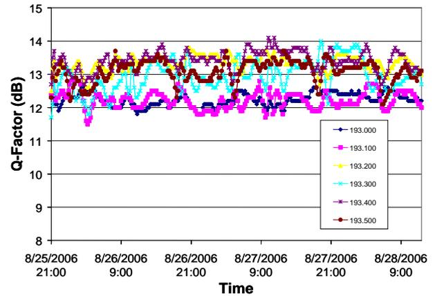
Figure 4. Measured Q performance of the initial 6x10Gb/s CRZ OOK channels on the upgraded express 11,000 km DLS. The insert shows frequencies in THz.
