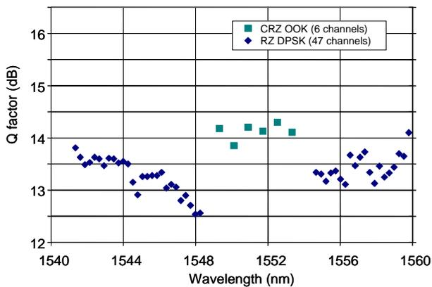
Figure 3. Simulated mean Q performance of an upgraded express 11,000 km DLS.
