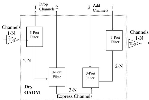
Figure 5. A simple implementation of OADM using 3-port channel selection filters.
