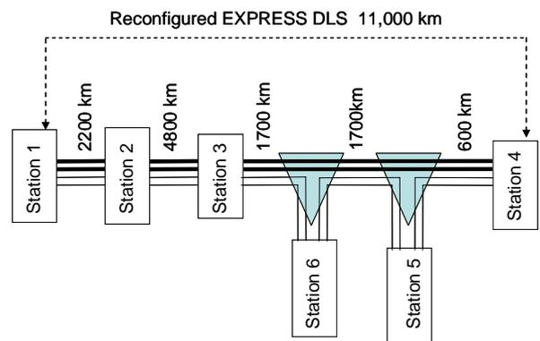
Figure 2. Schematics of an upgrade involving network reconfiguration from local DLSs to 11,000km express DLS connecting stations 1 and 4. The bold line indicates the reconfigures express DLS.
