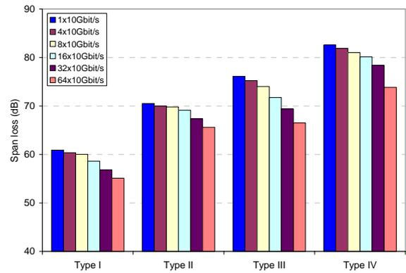
Figure 2: System reach of various repeaterless topologies shown for a range of capacities. The simulations assumed moderate effective area fiber ( $80\mu m^2$ ), RZ-DPSK modulation format and single wavelength Raman pumps where applicable.
