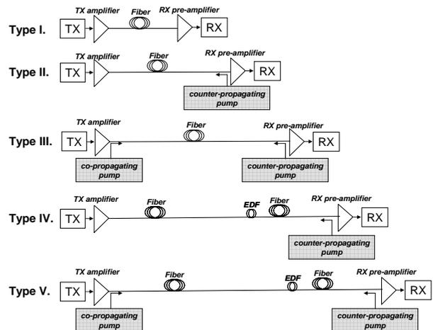
Figure 1. Main topologies used in repeaterless design. The types are arranged in order of increasing complexity. Type I has the shortest reach and Type V has the longest reach.
