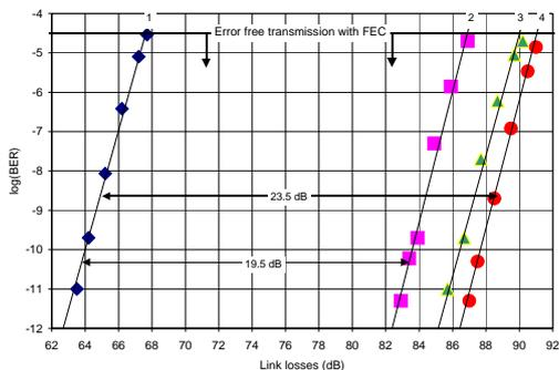
Figure 3: BER measurements vs. link losses. 1.-without ROPAs, 2. only Rx ROPA at optima position, 3&4.- with Tx ROPA placed at 35.75 and 50.75 km from the pump source.
