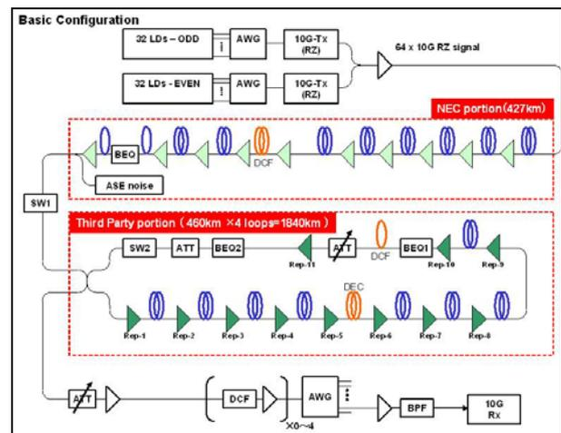
Figure 2 Diagram of Looped Test-bed
