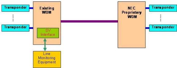
Figure 3 The Monitoring Scheme for the existing and new wet plant
