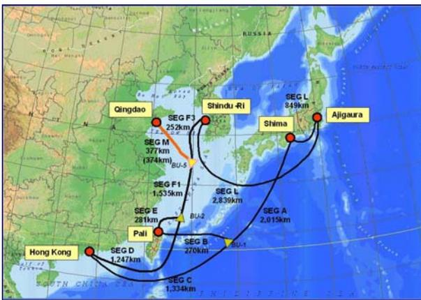
Figure 1 Route Map for EAC1 Qingdao Landing Extension
