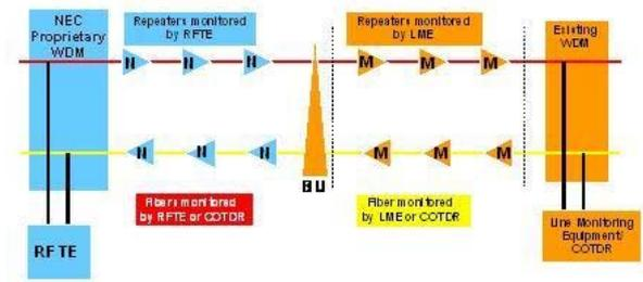
Figure 4 Wet Plant Monitoring Scheme
