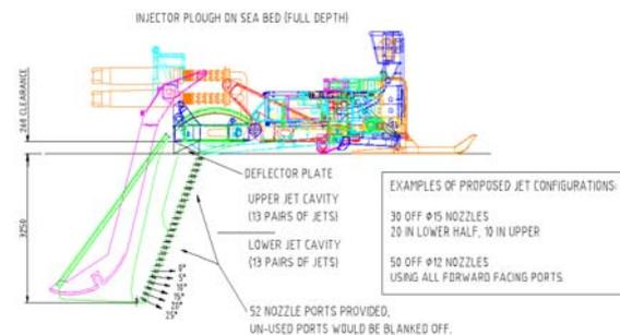
Figure 9 3m Burial “High Plough Injector”
