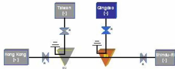
Figure 5 Power Feeding Configuration
