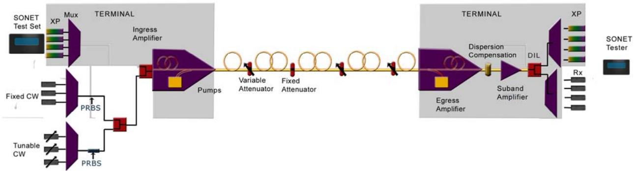
Figure 1. Set-up of the emulated link
