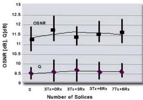
Figure 5: Impact on performance of point losses in shore-end sections
