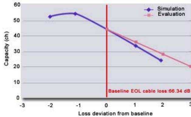
Figure 3. Capacity vs. Loss Devtion from the Baseline
