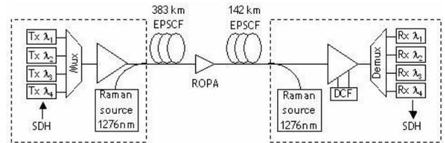
Figure 3: Experimental set-up for 525 km transmission
