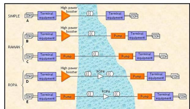
Figure 1: Optical amplification configurations
