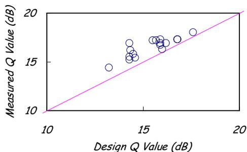
Figure 3 An example of estimated Q values vs actual measured Q values of upgraded 10Gb/s DWDM system
