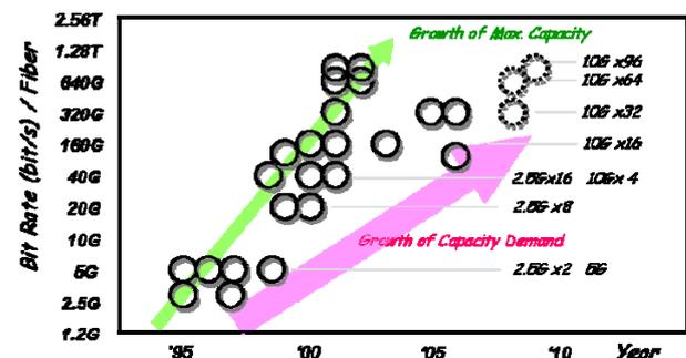
Figure 1 Growth of maximum capacity per fiber pair on constructed optical amplified submarine repeater systems
