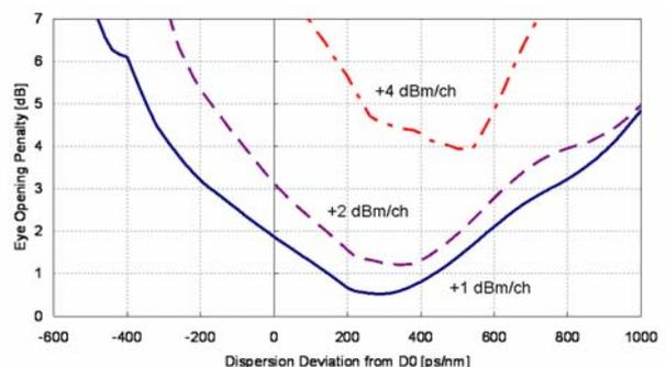
Figure 2 An example of simulation results for upgrading an existing 2,600km system with 10Gb/s DWDM
