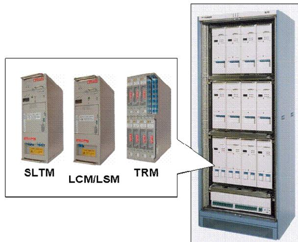
Figure 4 Submarine Line Terminal Equipment (SLTE)
