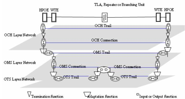
Figure 4 - Optical Transport Layer Networks
