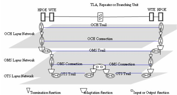
Figure 4 - Optical Transport Layer Networks
