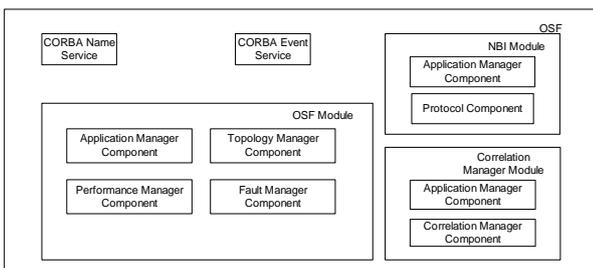
Figure 3 - OSF Architecture
