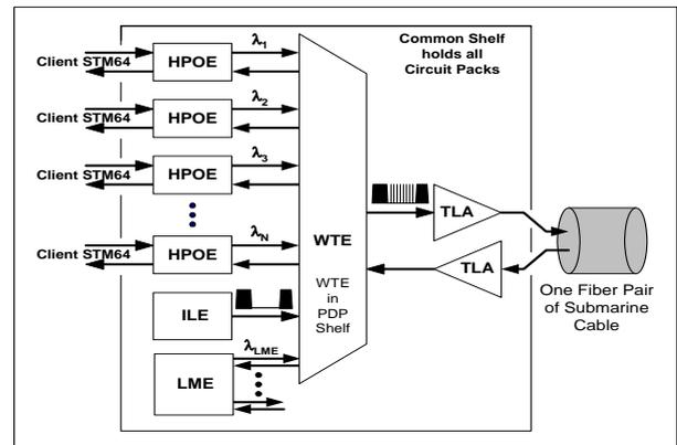
Figure 1: Architecture of complete Submarine Line Terminal Equipment
