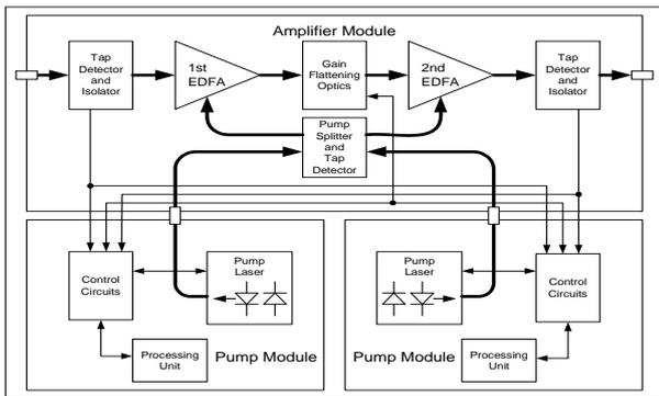
Figure 4: TLA Block Diagram
