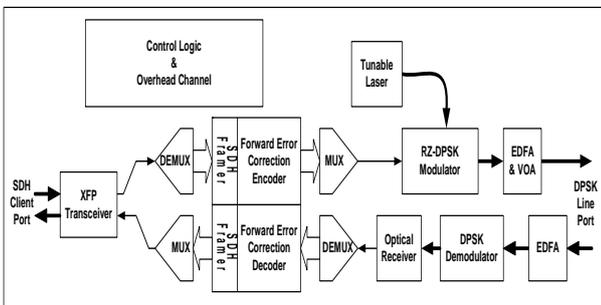
Figure 2: Transponder Block Diagram
