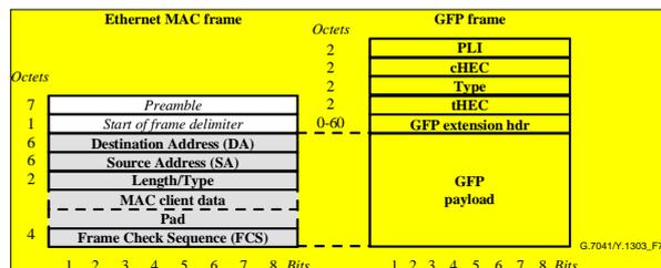
Figure 2. : GFP-F Mapping (G.7041) for Ethernet Signals
