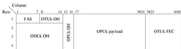
Figure 1: OTUk Frame Structure
