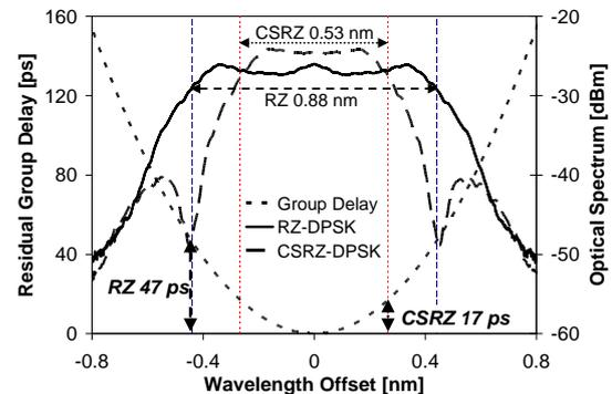
Figure 1: Residual group delay (after dispersion compensation) after 6,250 km, and optical spectra for RZ-DPSK and CSRZ-DPSK [1].
