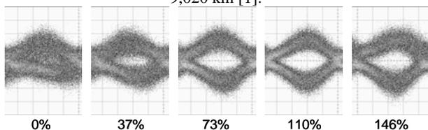
Figure 2b: Balanced eye diagrams for the RZ-DPSK format with different slope compensation ratios. [1]
