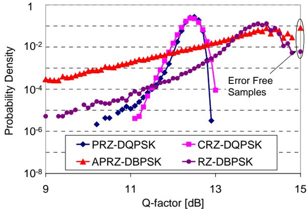
Figure 3: Long term Q-factor distributions for 4 modulation formats. [10]
