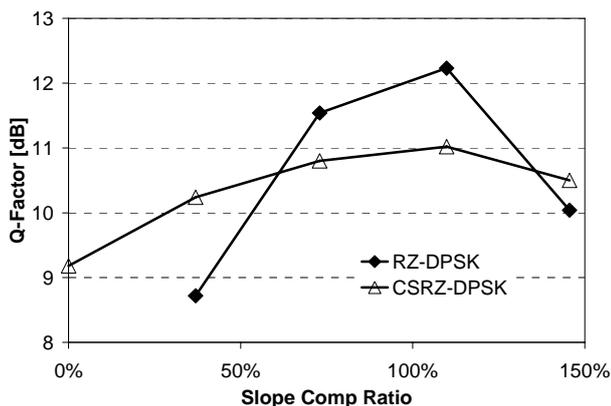
Figure 2a: Q-factor vs. slope compensation ratio after 9,020 km [1].
