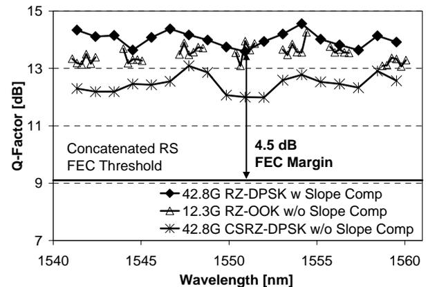
Figure 4: Q-factors for 42.8 Gb/s RZ-DPSK (w/ slope compensation), 42.8 Gb/s CSRZ-DPSK (w/o slope comp.), and 12.3 Gb/s RZ-OOK [1].
