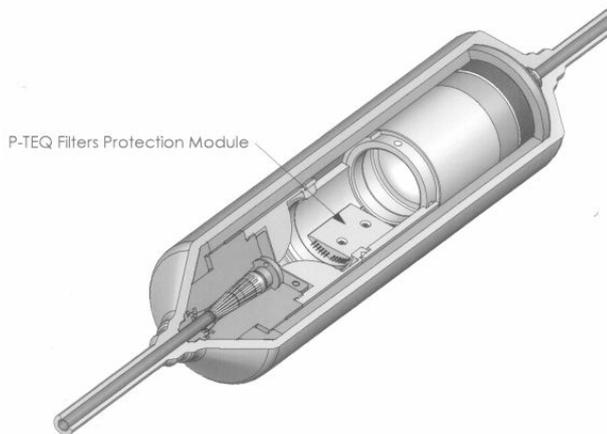
Figure #1. P-TEQ Joint Box 3D View
