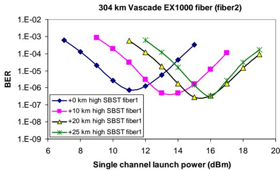
Figure 5: Transmission results for single channel launched into unrepeated spans comprised of various lengths of high SBS-threshold G.652-compliant fiber (fiber1) and 304 km Vascade EX1000 fiber (fiber2).
