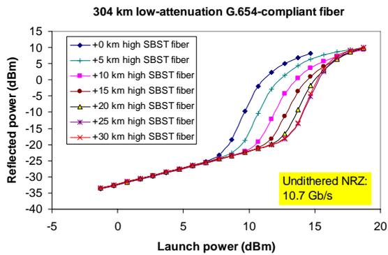
Figure 1: Experimental results for SBS reflected power for a span comprised of varying lengths of high SBS-threshold fiber plus 304 km of low-attenuation G.654-compliant fiber.
