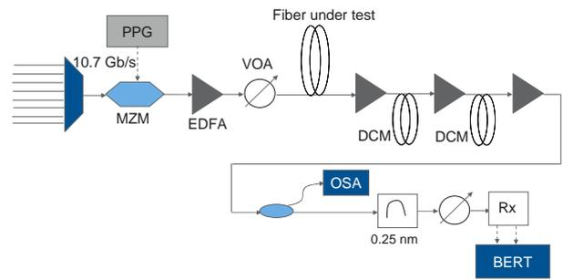
Figure 4: Schematic diagram of transmission system test setup.
