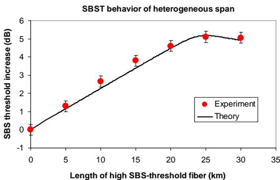
Figure 3: Model prediction and experimental results for increase in SBS threshold as a function of the length of high SBS-threshold fiber (fiber1) at the span input of a heterogeneous span comprised of fiber1 plus 304 km of the G.654-compliant fiber (fiber2)
