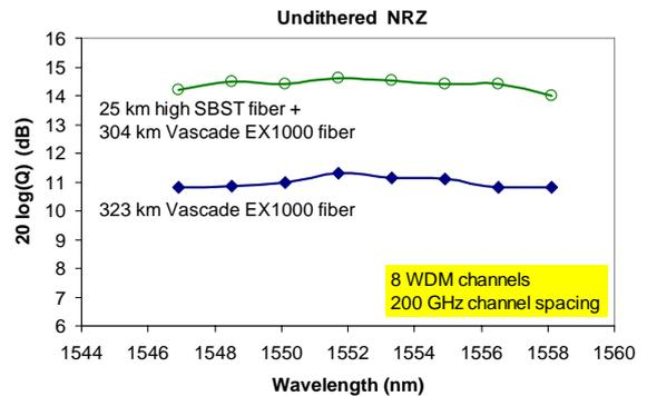
Figure 7: Q values calculated from measured BER data for the 8-channel WDM systems transmitted over a 323 km homogeneous span and a 329 km heterogeneous span.
