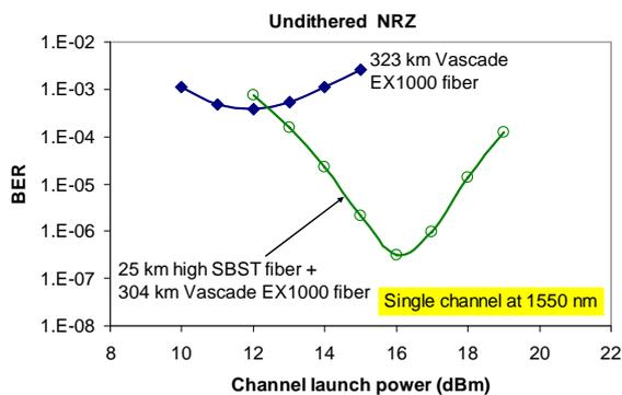
Figure 6: Experimental results comparing single channel transmission through approximately comparable length homogeneous and heterogeneous spans.
