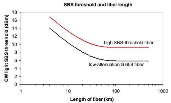
Figure 2: Theoretical model dependence of SBS threshold on length of fiber for two fiber types.
