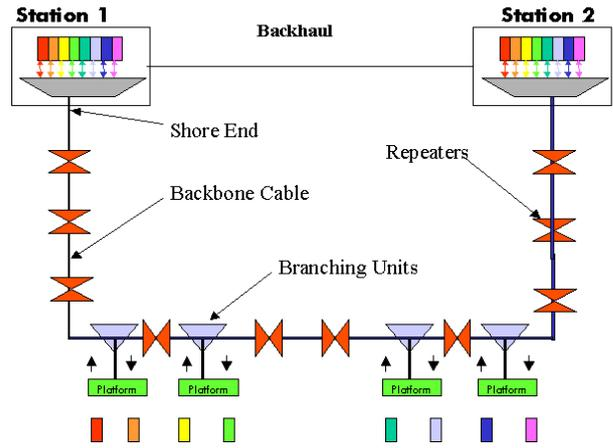
Figure 6: Connectivity on a per wavelength basis.
