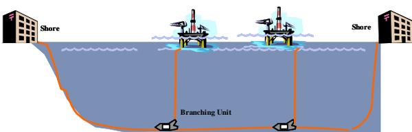
Figure 3: Unrepeated network with spur to the hub
