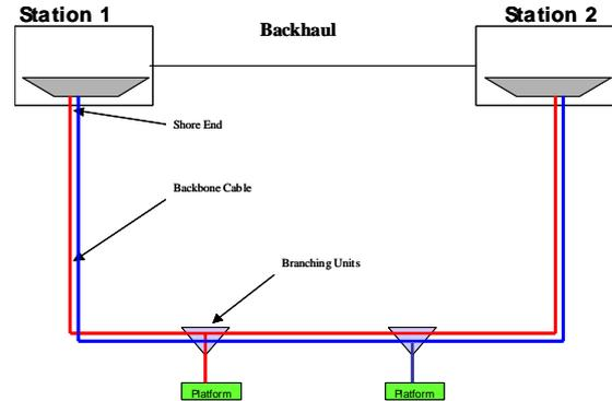
Figure 4: Connectivity on a fiber pair basis
